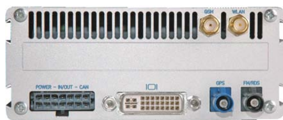
Base unit rear panel connections (rectangle shows available area for custom connections)
