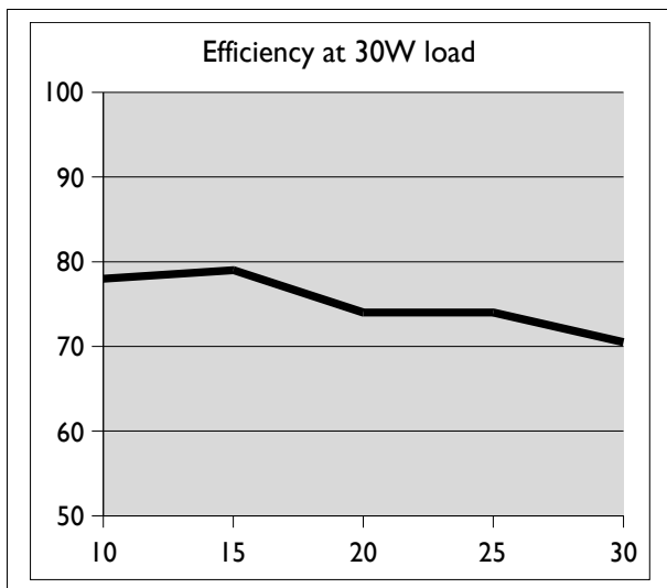
Typical performance curve with a evenly distributed load. 5VSB/0.75A, 3.3V/1.5A, 5V/2.5A, 12V/0.8A.
